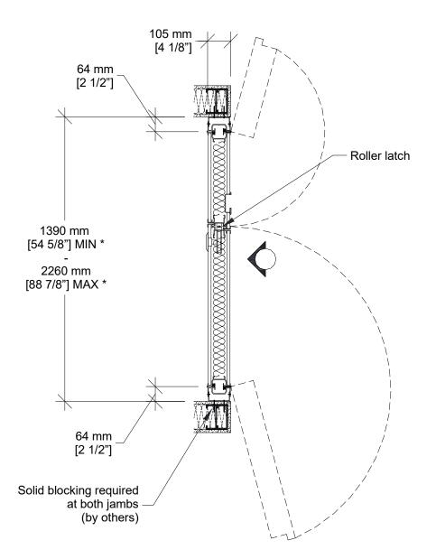
\* Min/Max dimensions are fabrication limits and do not account for job-specific conditions.
